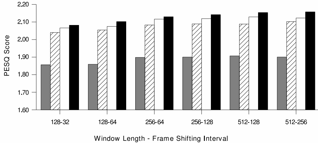
Figure 6.6. Effects of microphone spacing on the PMBSS method. Gray bar: 1 cm spacing, dashed bar: 2 cm spacing, white bar: 3 cm spacing, black bar: 4 cm spacing.
